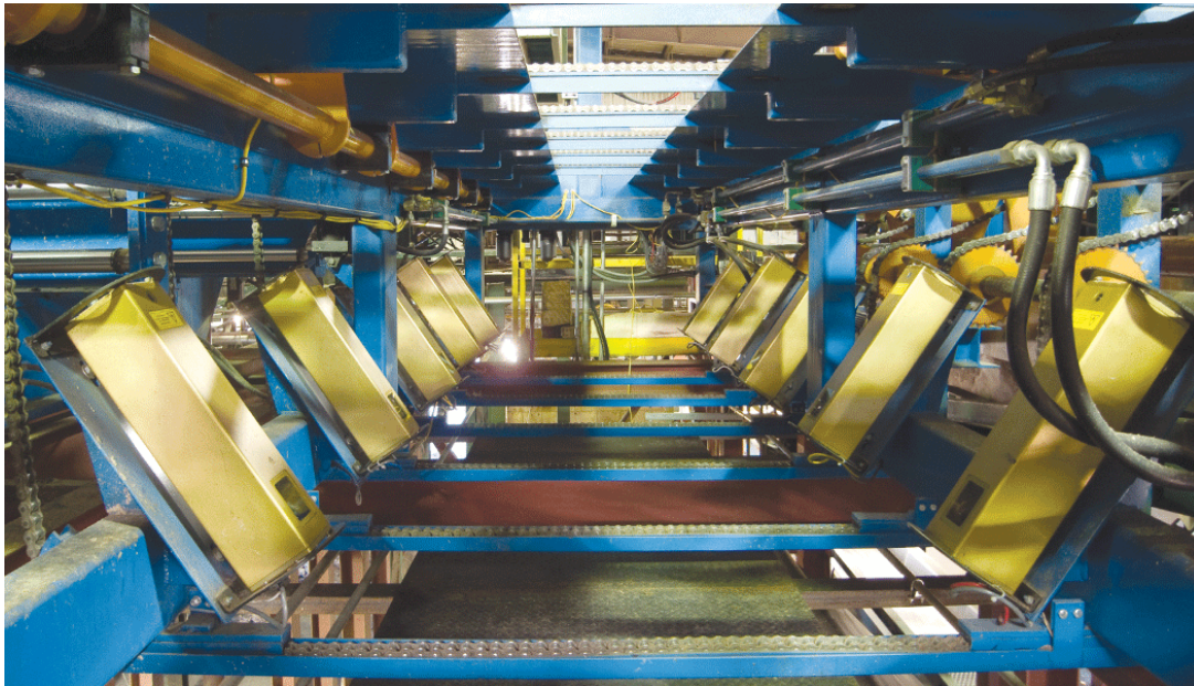
Scanners with shorter standoff distances provide more flexibility when placing banks below conveyance systems.
